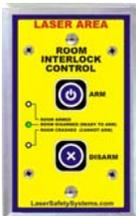
The Interlock Control Module is used for arming and disarming the laser interlock system. One or more interlock control modules can be placed anywhere within a single laser area to control the state of the interlock. The “DISARM” button will always take precedence over a request to arm the system. (All crash switches also override ability to arm the system.)
