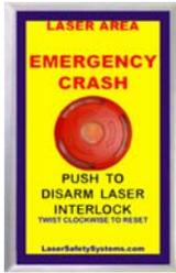
The EMERGENCY CRASH MODULE is a safety device specified in ANSI Z136.1-2007 section 4.3.10.2.1. It should be placed in a location quickly accessible to the laser workers and it is intended to be used for emergency deactivation of the laser or laser shutter to reduce the output levels at or below the applicable MPE.
